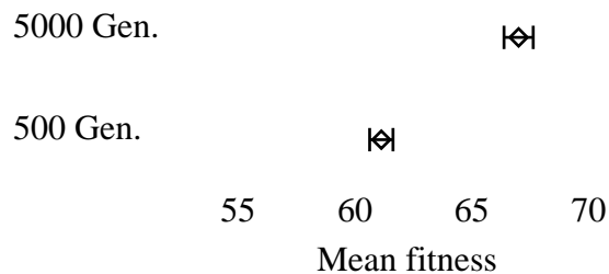
Figure 7: Graphical 95% confidence interval for mean fitnesses of more evolved and less evolved robots. These intervals are based on comparison of 2 sets of 400 paint bots.
